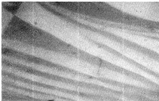
FIG. 3. Metastable anisotropic texture in a 25-layer film at T = 48.06^\circ\text{C} .
