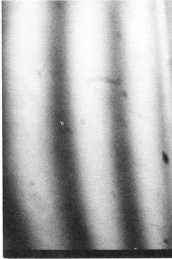
FIG. 5. Striped state of the plane director field of the smectic- C^* phase in an N=400 film of chiral C7 .
